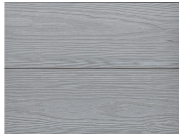
FAEN - KEBONY WEATHERED EXTERIOR INSTALL (NO TOP COAT REAPPLIED)
