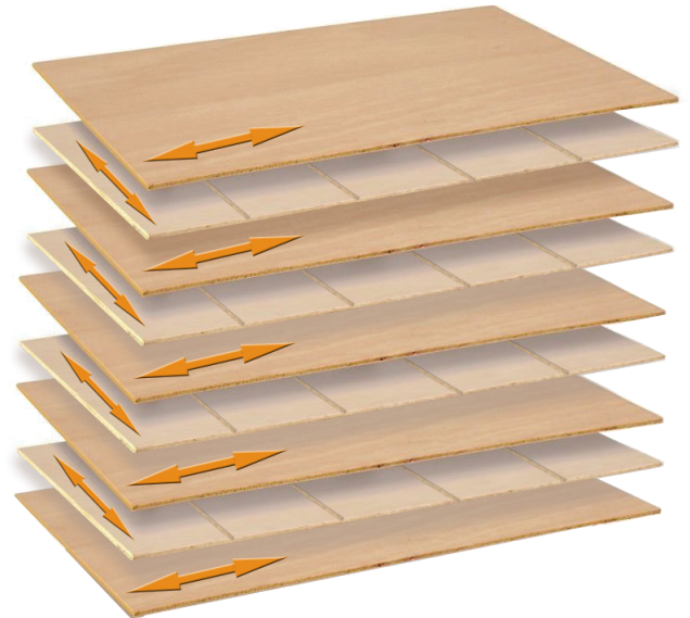
Fig. 1.3 – Cross-Grain Configuration – The cross-grain layering of engineered wood is what enhances its stability.
