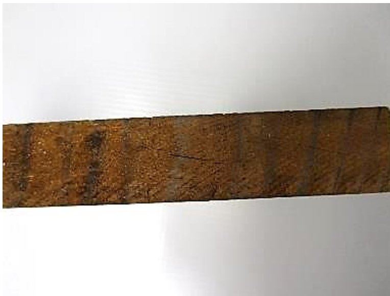
Photo No. 8 Typical Post-Test Edge Cracking Detail
