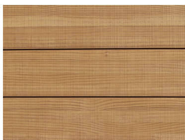
NATURAL EXTERIOR CLADDING (WEATHERED 2 MONTHS)
