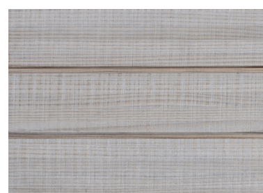
PATINA EXTERIOR CLADDING (WEATHERED 2 MONTHS)
