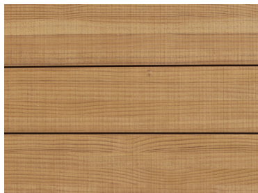
NATURAL EXTERIOR CLADDING (WEATHERED 2 MONTHS)
