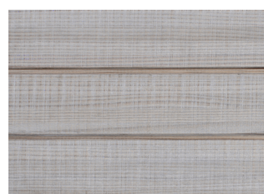
PATINA EXTERIOR CLADDING (WEATHERED 2 MONTHS)
